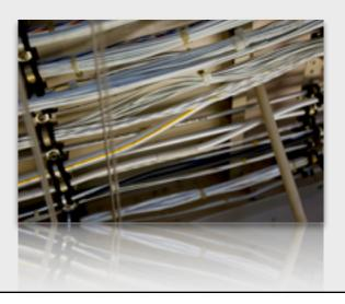
The leads may be improperly identified or missing labels, according to the FAA's proposed airworthiness directive to remedy the situation.
